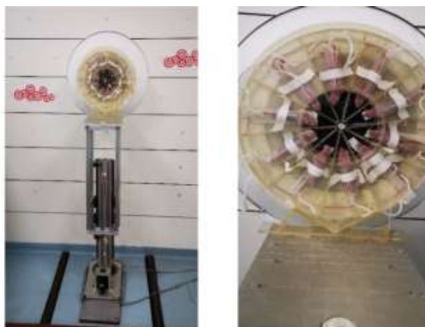
The situation of the mice model exposed to thermal neutron irradiation for BNCT experiments in vivo
