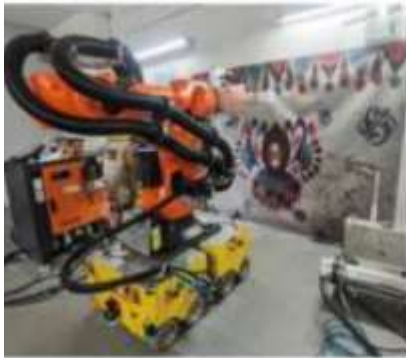
Mobile electron beam equipment designed for sterilization of murals and organic cultural relics
